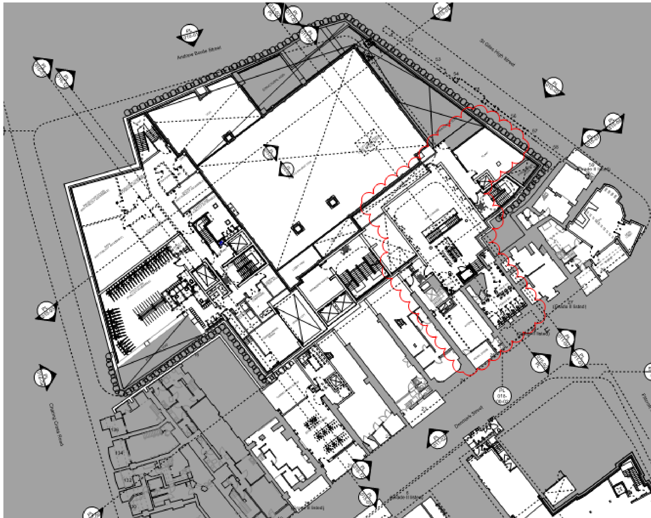
Above: Proposed Lower Ground Floor Plan (new basement under no. 23, structural voids under 22 and 25 reworked)
