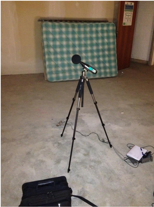
Figure 4 Photograph showing the set up for simultaneous noise and vibration measurements
