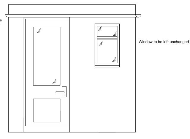
Replacement of rear timber door with single glazing for timber door of identical design with double glazing, to be carried out by appropriate craftsman
