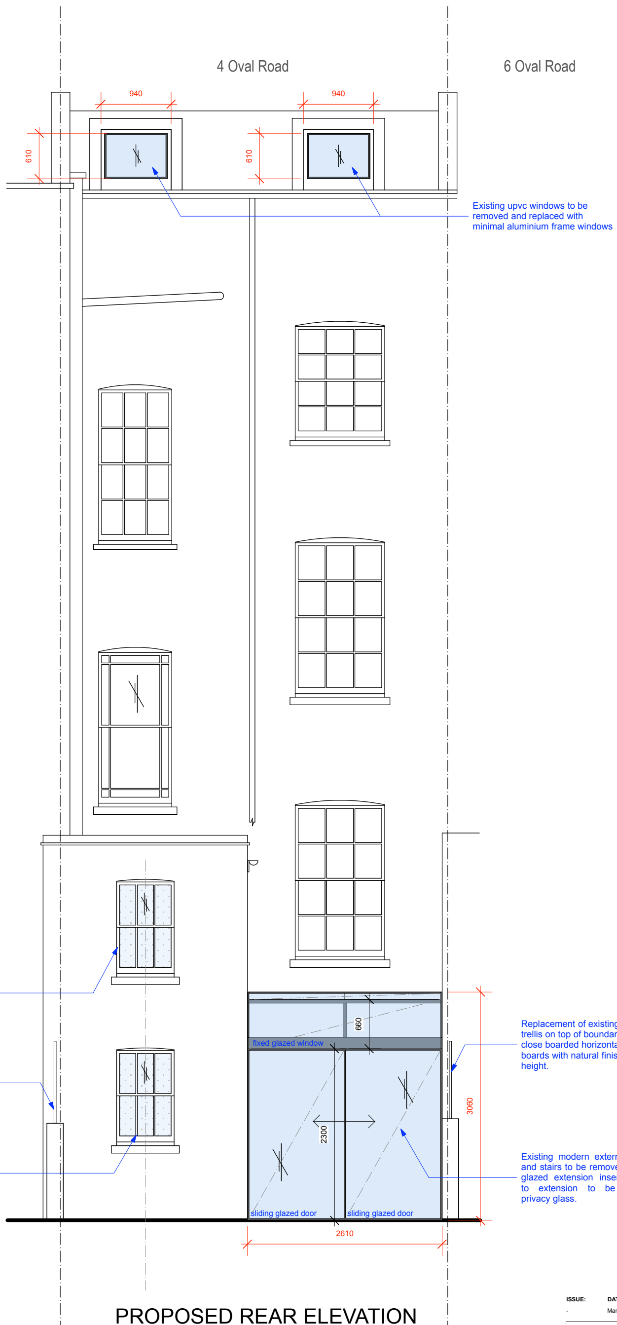
1 PROPOSED REAR ELEVATION Scale: 1:50
