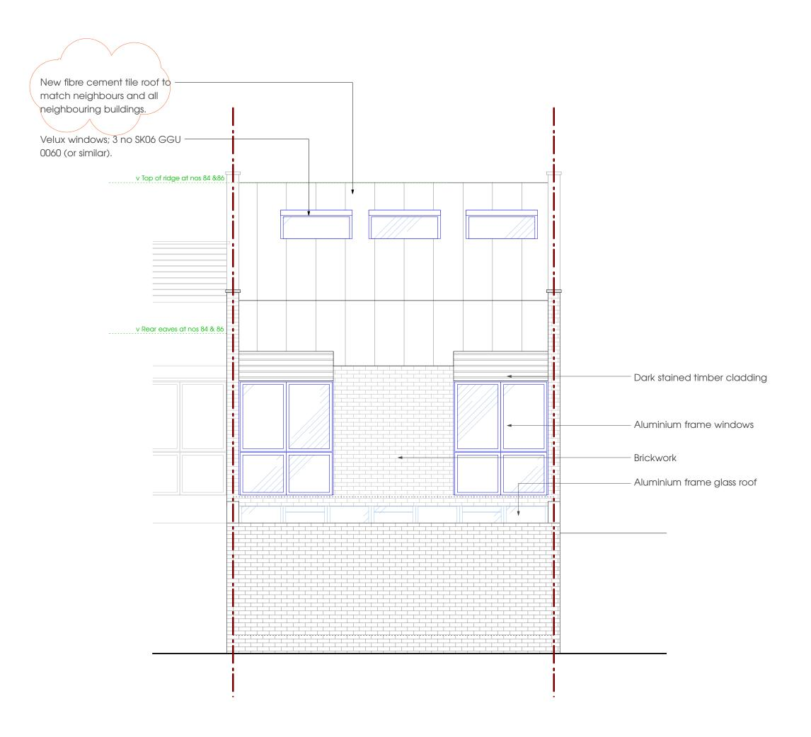
DRAWING Proposed rear elevation
