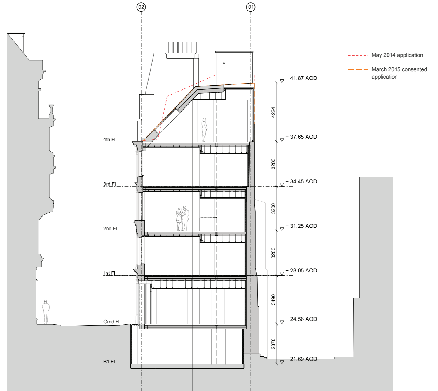
▲ Section 01: Proposed 4th floor extension with extents of refused scheme (May 2014) in red and the consented scheme (March 2015) in orange.
