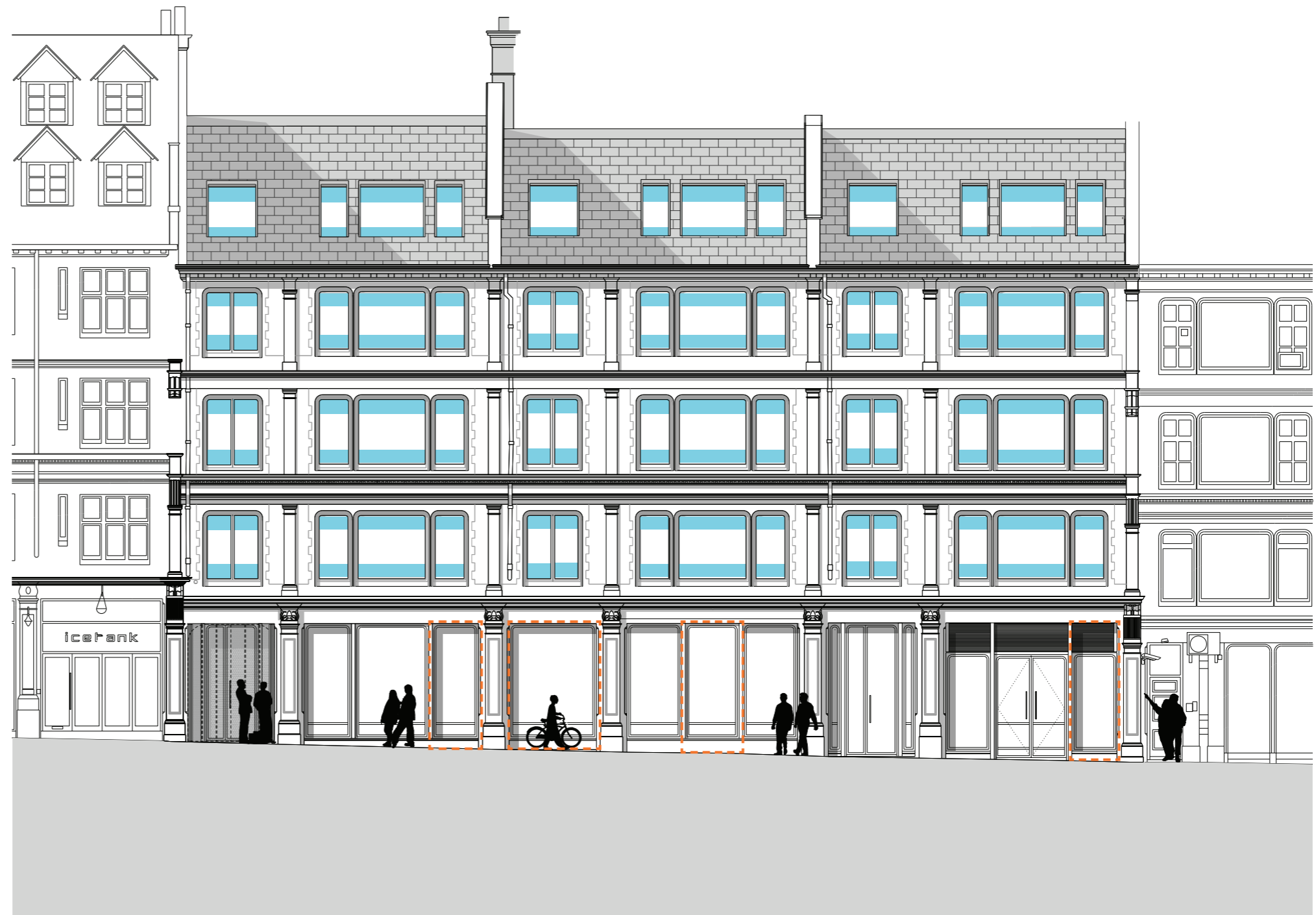
▲ Elevation illustrating the alterations to the design; the orange lines show the March 2015 consented ground level doors, which have been omitted from this proposal.
