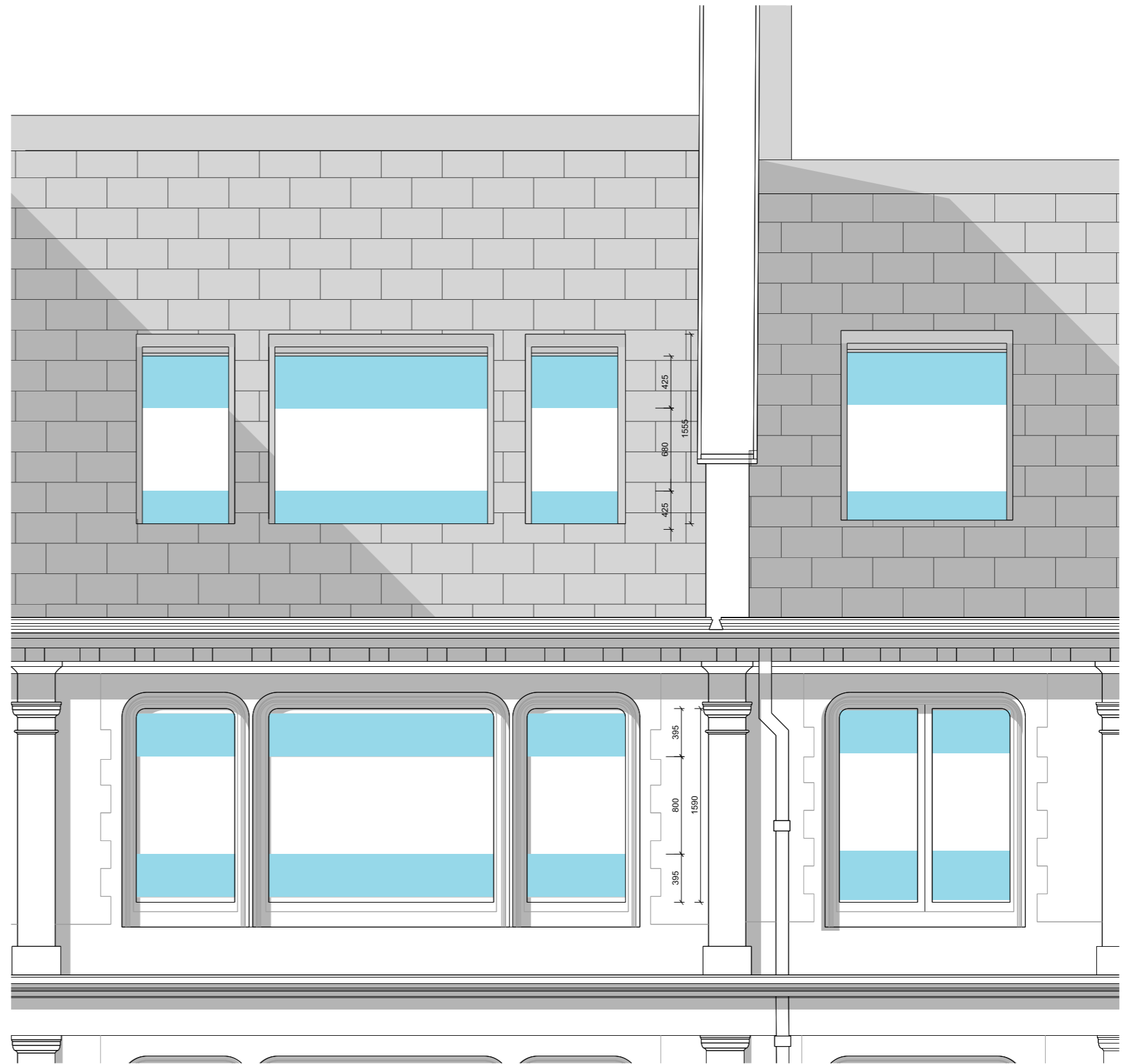
▲ Detail elevation illustrating the sizing of fritted and untreated glass
