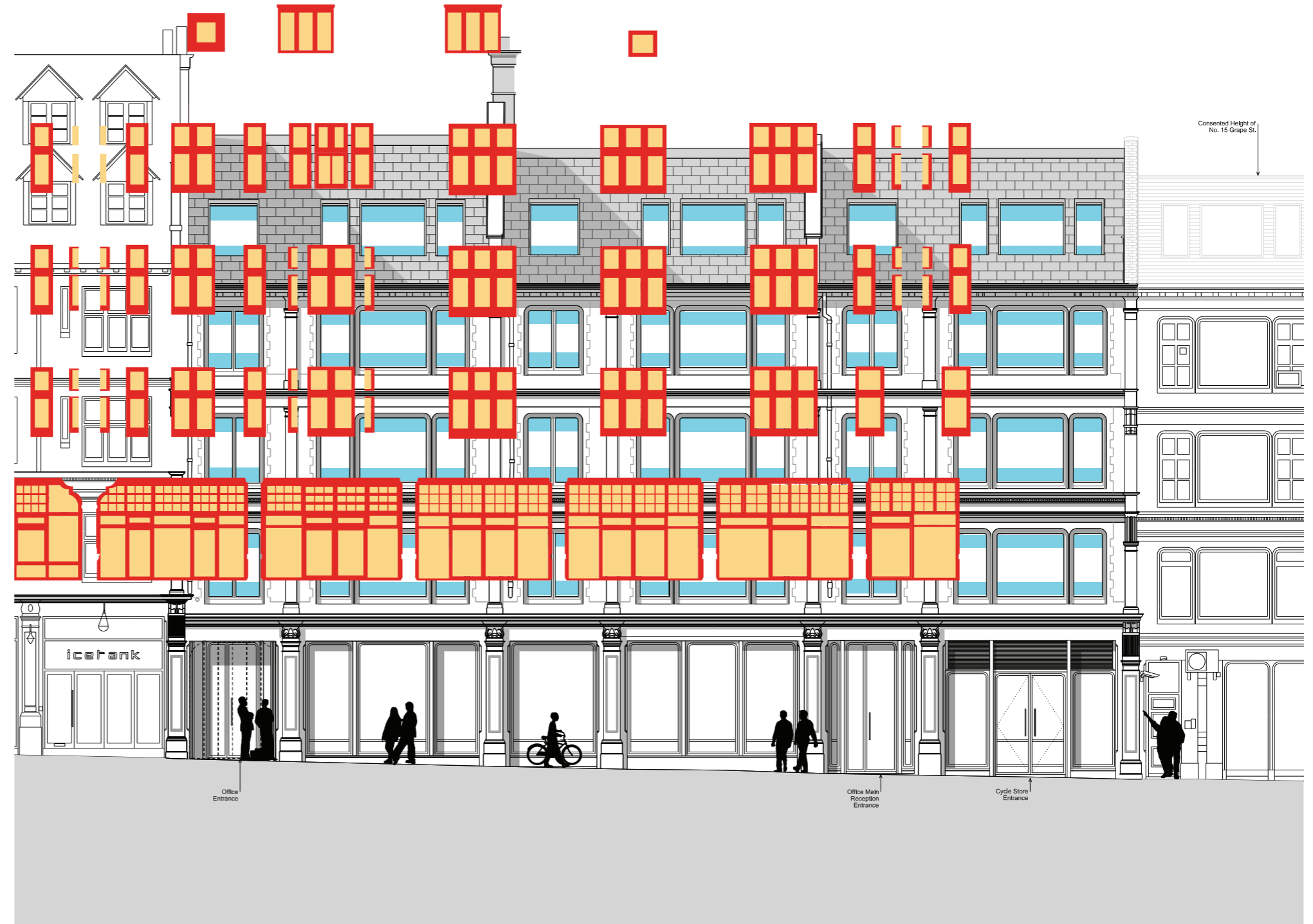
▲ Elevation illustrating zone of fritted glazing in relation to the KEM window locations
