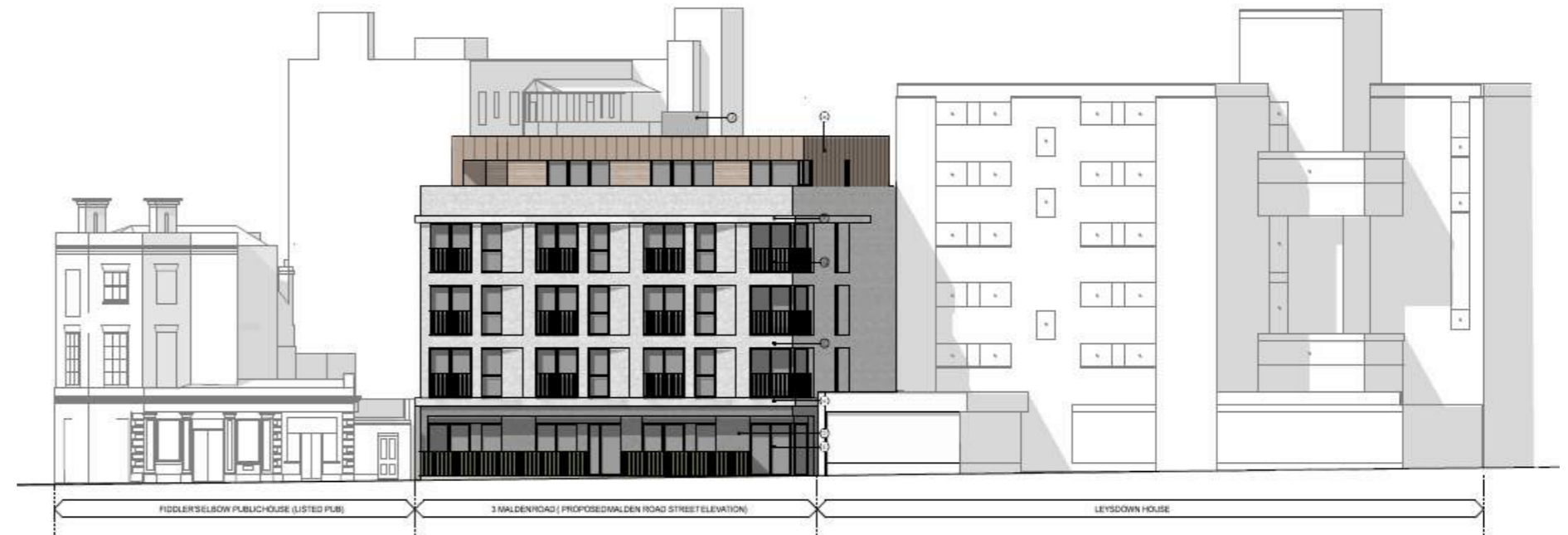
Figure 23: East elevation along Malden Road showing relationship of proposed building to the Fiddler's Elbow Public House. Critically, there will be minimal intervention to the southern Site boundary; limited to the ground floor only and adjoining a later extension of the statutorily listed building. This elevation reintroduces a verticality and rhythm to the streetscene as
