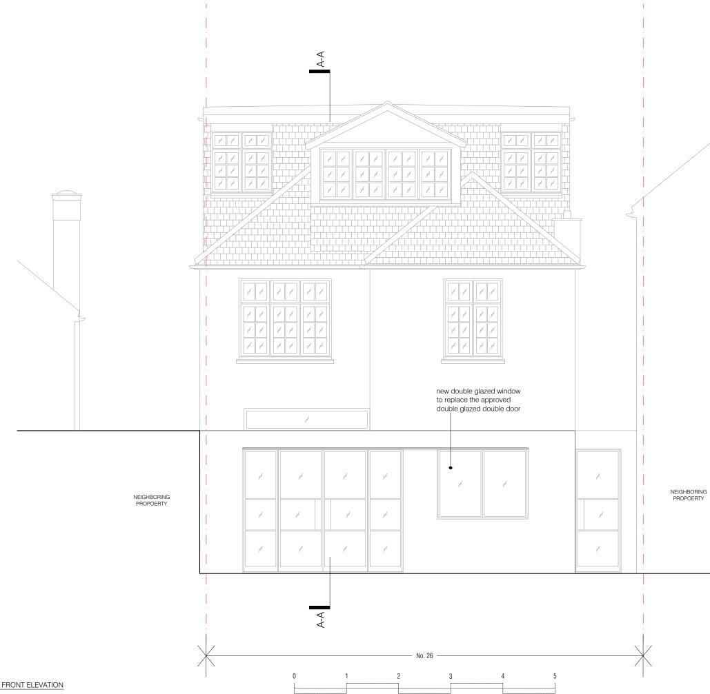
$01 \; \tfrac{\text{NEW PROPOSED FRONT ELEVATION}}{\text{scale 1:50}}$
