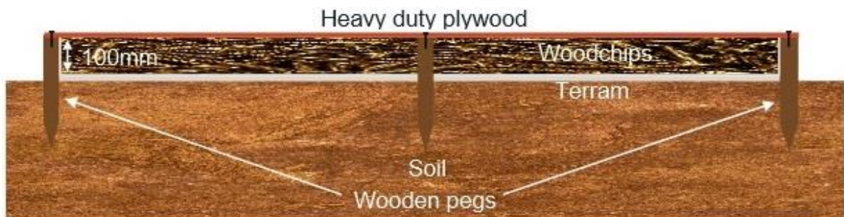
Figure 7. Plywood sheeting used as ground protection.
