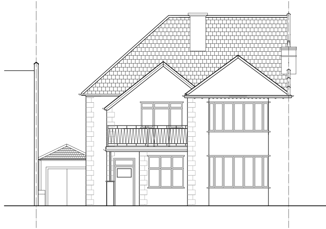
EXISTING FRONT ELEVATION
