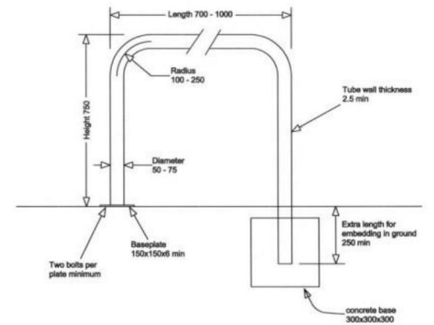
Surface fixing mode      Ground embedding mode
