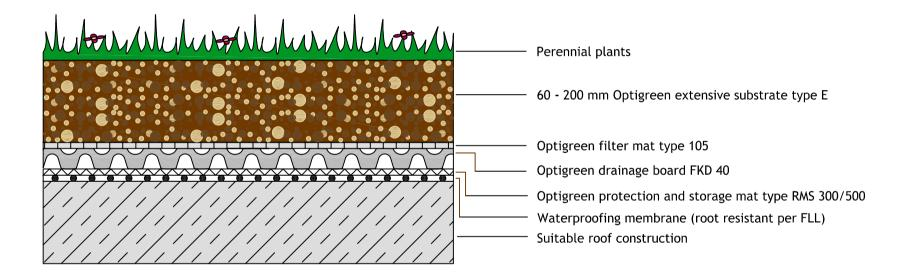
The depicted product solution is intended for use with green roof systems. Other construction tradework is simplified in this representation and should be constructed according to current industry standards. This drawing is not to scale. Optigreen reserves the right to make changes to its product solutions.
