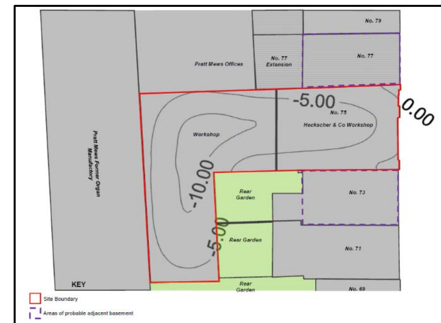
Figure (m) Long Term Ground Movement Contours (from LBH's ground movement assessment)
