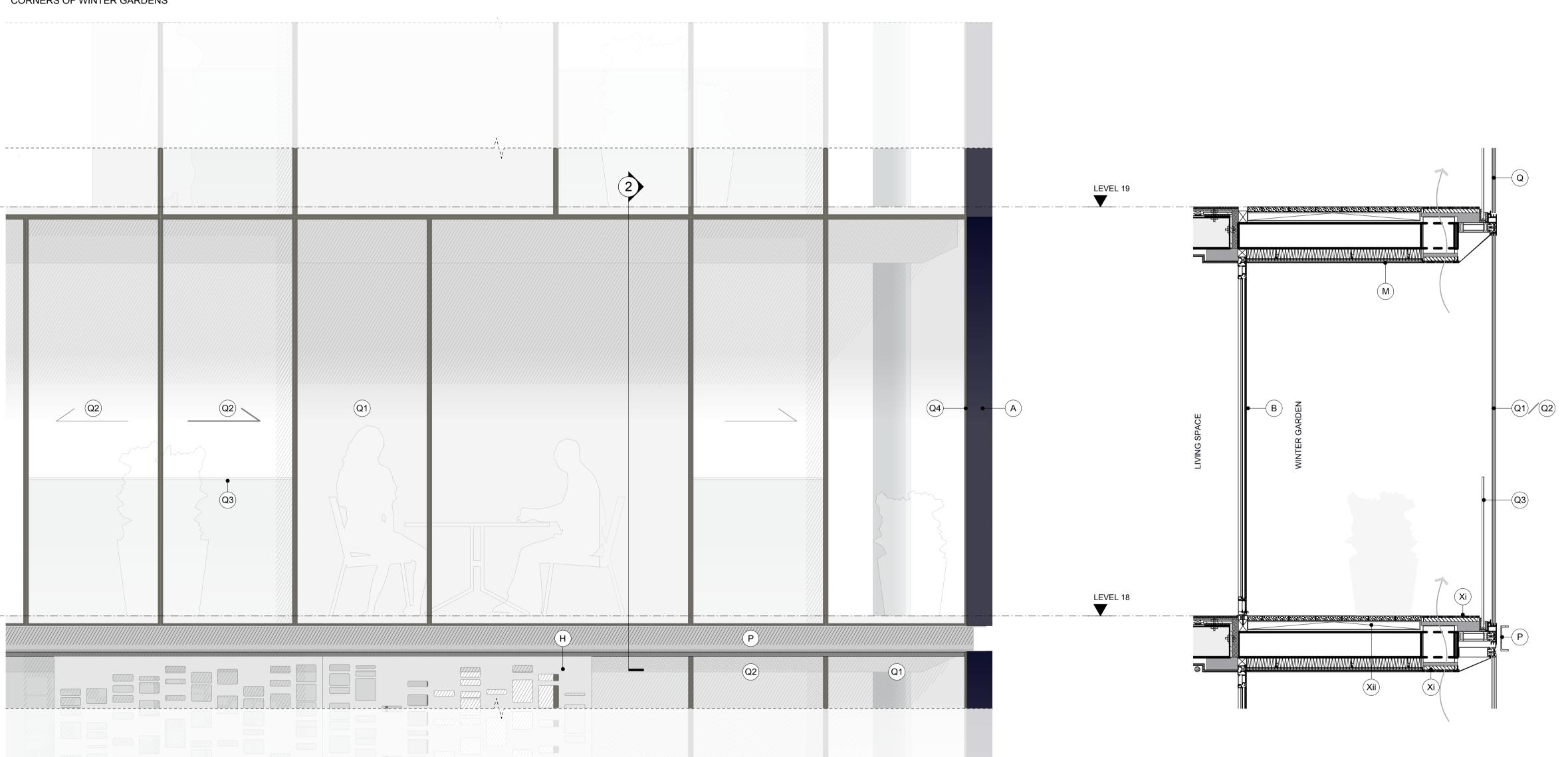
UNITISED FRAMELESS CURTAIN WALLING SYSTEM WITH CIRCA 200M DEEP GLASS RAINSCREEN FIXED TO OUTSIDE. RAL 5011 STEEL BLUE CERAMIC FRIT TO REAR (FACE 2) OF RAINSCREEN GLASS. GLASS REVEALS AROUND EDGES (TOP, SIDES AND SOFFITS) OF OVERALL RAINSCREEN ZONE TO
