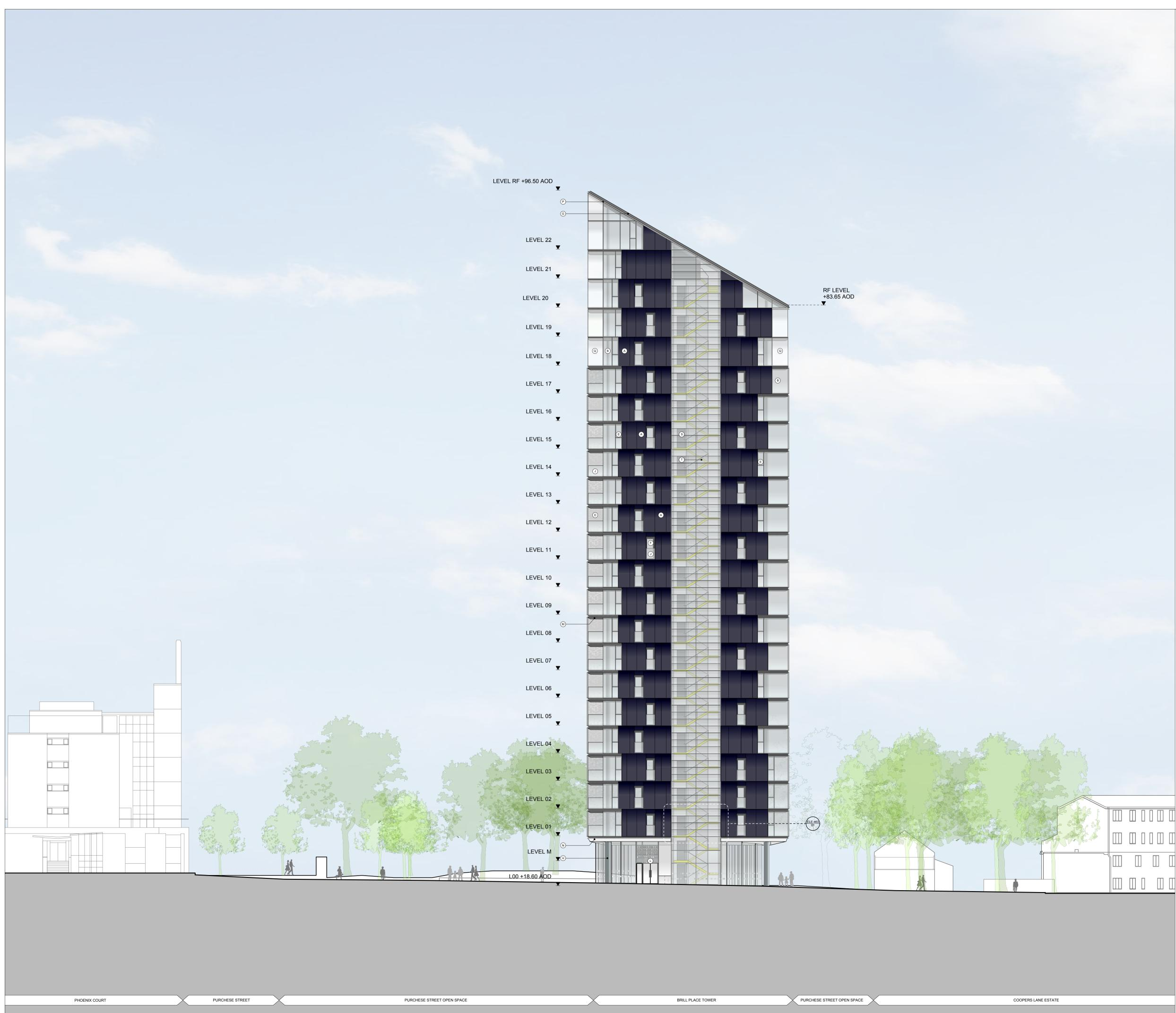
UNITISED FRAMELESS CURTAIN WALLING SYSTEM WITH CIRCA 200M DEEP GLASS RAINSCREEN FIXED TO OUTSIDE. RAL 5011 STEEL BLUE CERAMIC FRIT TO REAR (FACE 2) OF RAINSCREEN GLASS. GLASS REVEALS AROUND EDGES (TOP, SIDES AND SOFFITS) OF OVERALL RAINSCREEN ZONE TO MATCH
