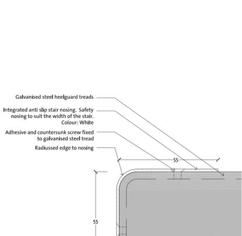
TYPICAL STAIR NOSING DETAIL - Scale 1:1
