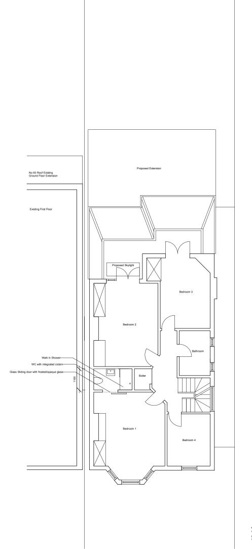
Proposed First Floor Plan Drawing Number 02\_02 scale 1:100,@A4 Rev A
