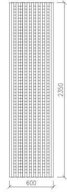
PMS - Privacy Metal Screens: Metal mesh (metal grating as per structure design and fixing to the building structure) All dimensions are indicative TBC as per site and supplier drawings.
