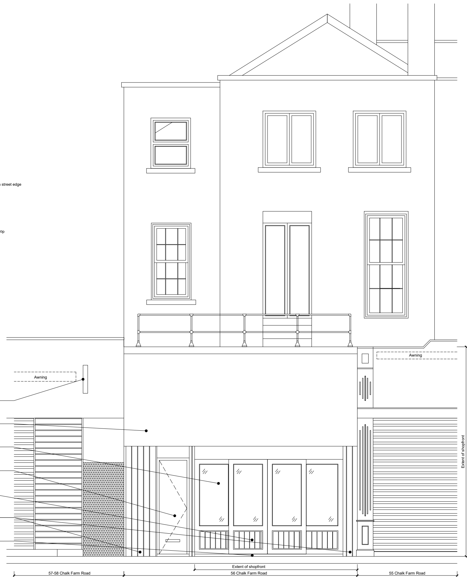
SHOP FRONT EXISTING ELEVATION
