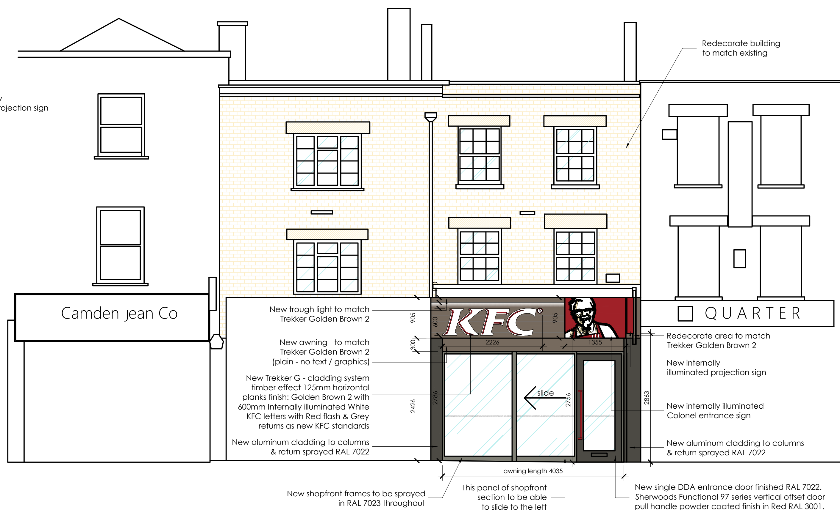
proposed shopfront elevation scale - 1:50 @ A1 / 1:100 @ A3
