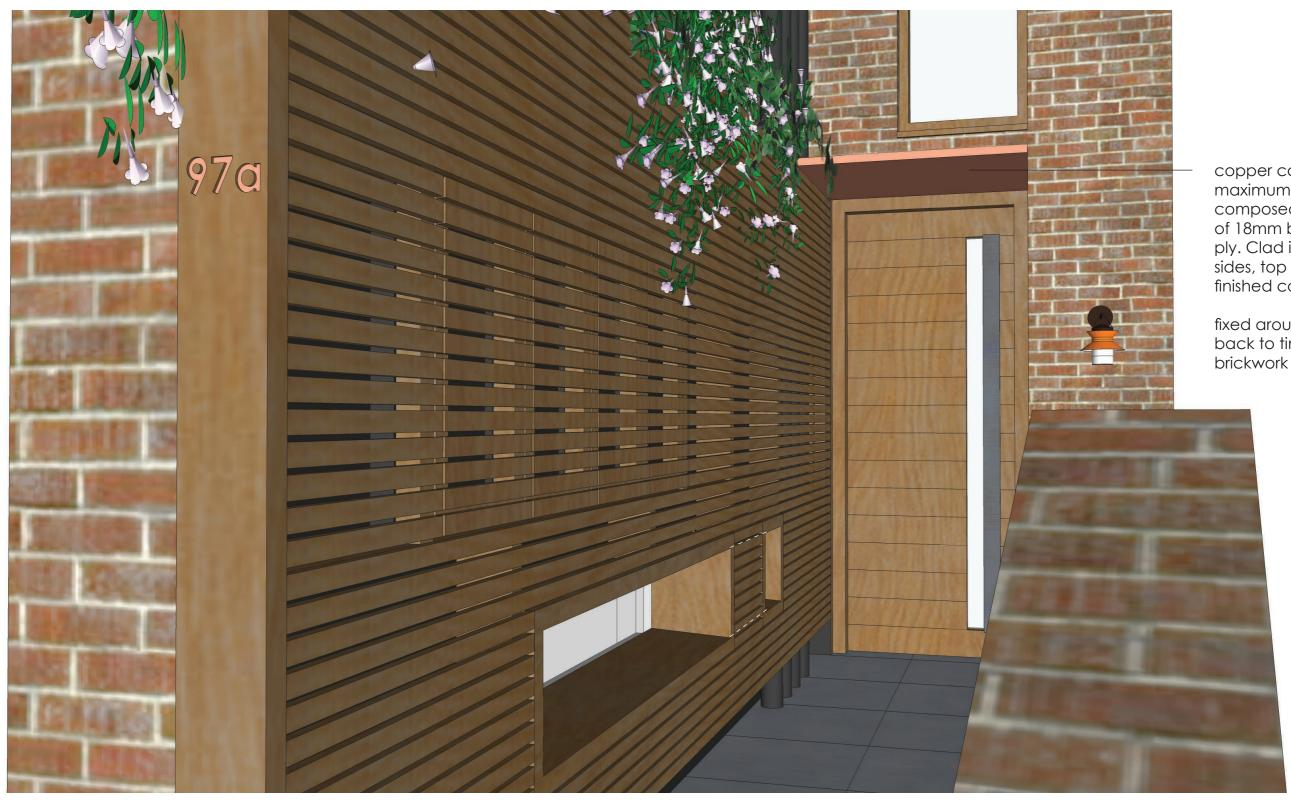
copper canopy (54mm maximum thickness) composed of three layers of 18mm bonded marine ply. Clad in copper on all sides, top and soffit with seal finished coat.
