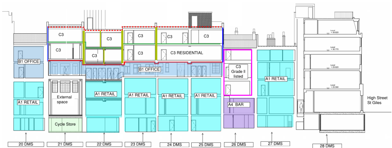
Figure 2. 21-26 Denmark St residential units typical section
