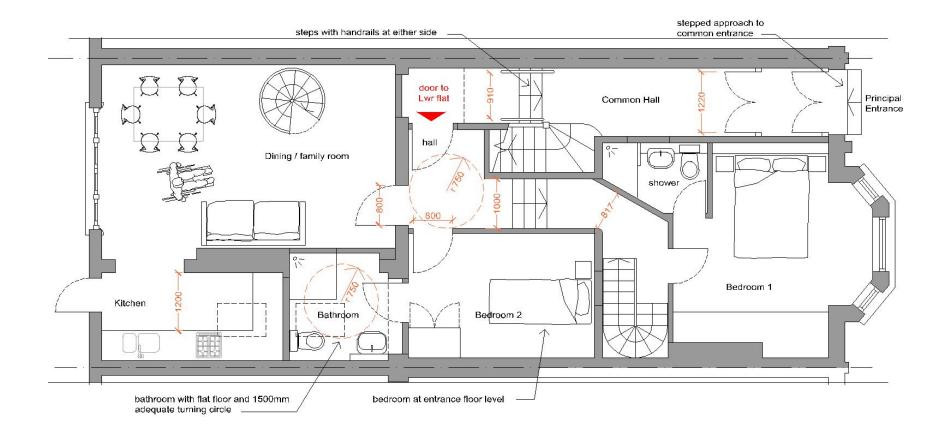
Diagrammatic layout of ground floor showing dimensions from Lifetime Homes Guidance
