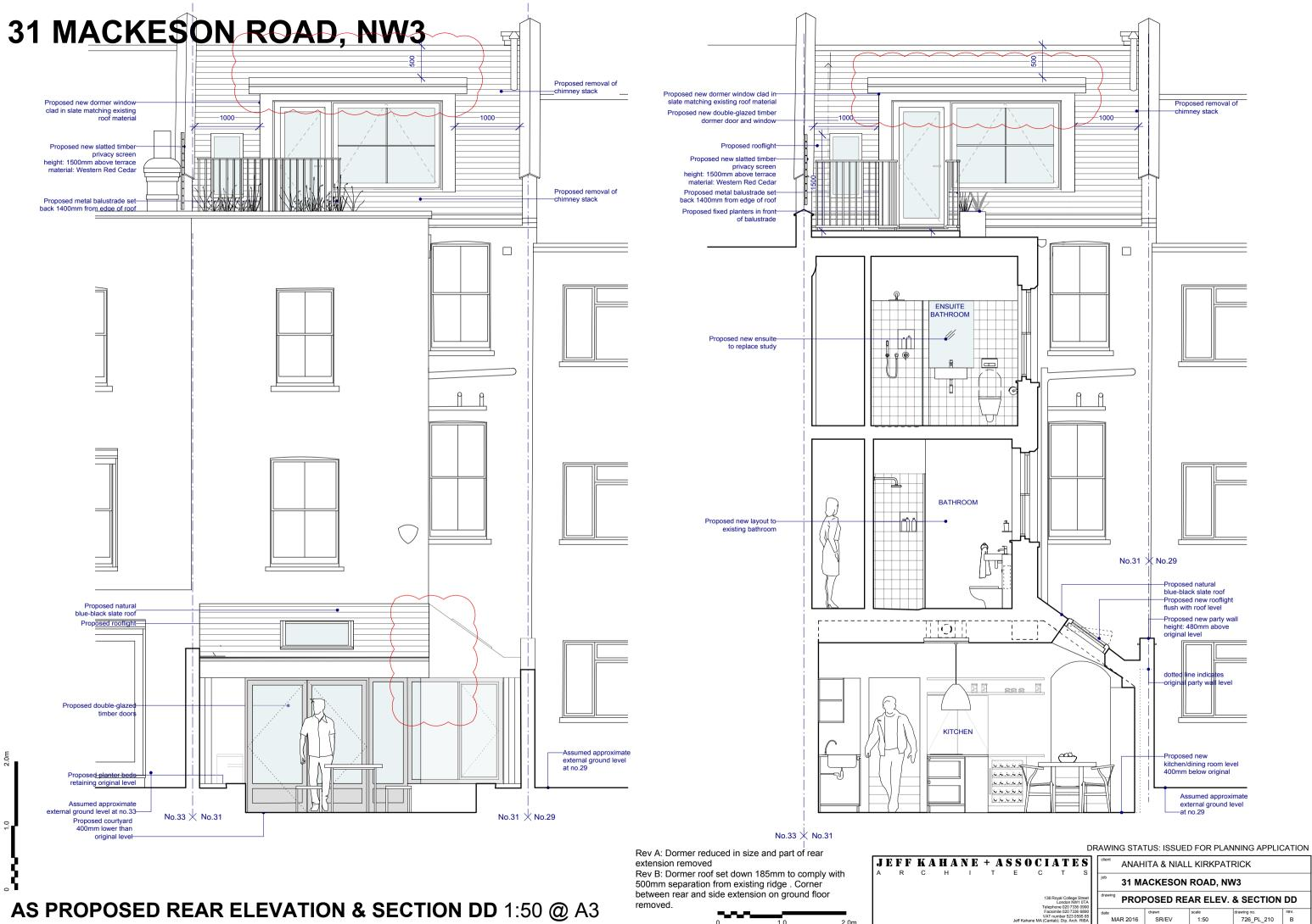
AS PROPOSED REAR ELEVATION & SECTION DD 1:50 @ A3
