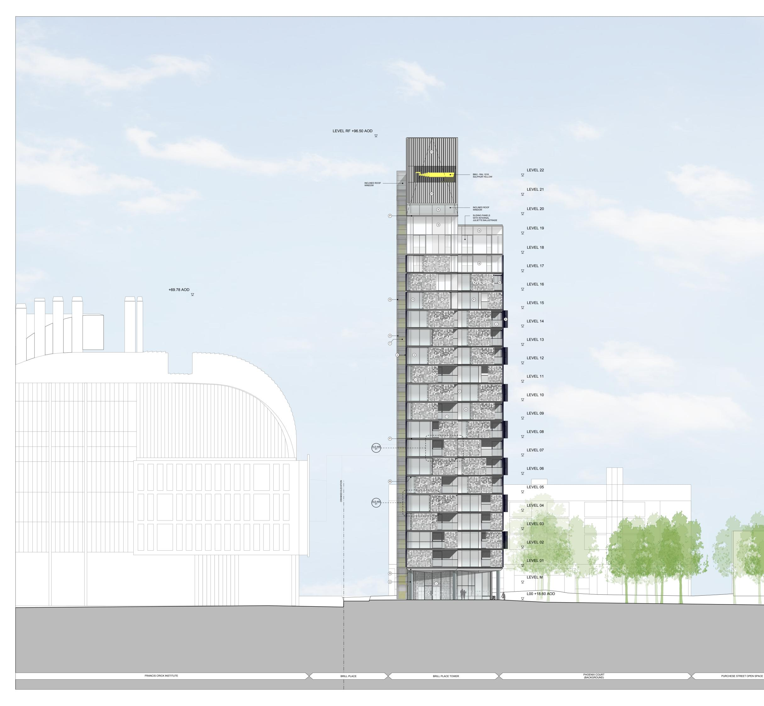
UNITISED FRAMELESS CURTAIN WALLING SYSTEM WITH CIRCA 200M DEEP GLASS RAINSCREEN FIXED TO OUTSIDE. RAL 5011 STEEL BLUE CERAMIC FRIT TO REAR (FACE 2) OF RAINSCREEN GLASS. GLASS REVEALS AROUND EDGES (TOP, SIDES AND SOFFITS) OF OVERALL
