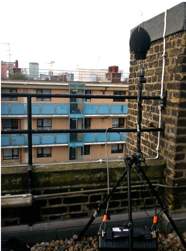
Figure 2 Sound level meter at unattended survey location L
