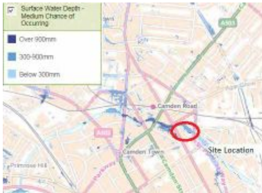
Figure 9: Surface water flooding (Environment Agency, 2015)
