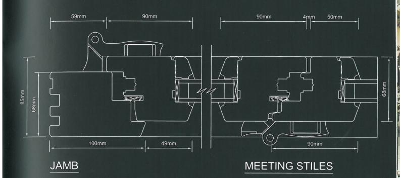
Standard Specification: Laminated larch, knot-free engineered (clear grade) timber from sustainable sources and complies with BS EN 942 2000. Hardwood cill sections.
