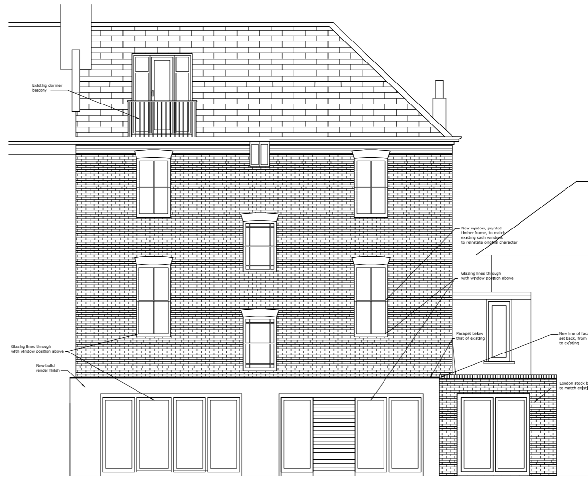
Fig 4.B PROPOSED View of rear elevation , note single sash window to replace four small windows. Large contemporary glazed doors line up with windows above.
