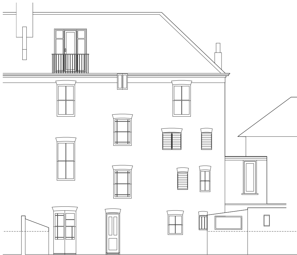
Fig 4.A EXISTING View of rear elevation , note four windows at first floor level, irregular openings on ground floor
