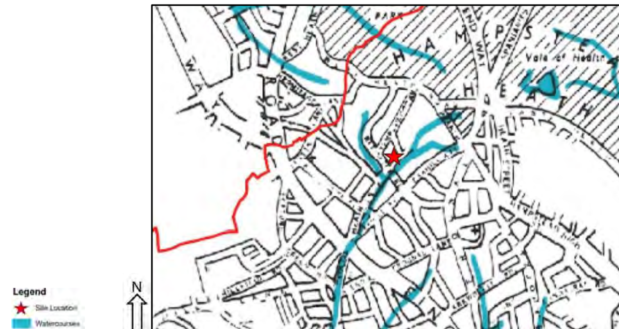
Figure (b) Subsurface Watercourses (Extract from Fig 11 of Camden Geological, Hydrogeological and Hydrological Study)
