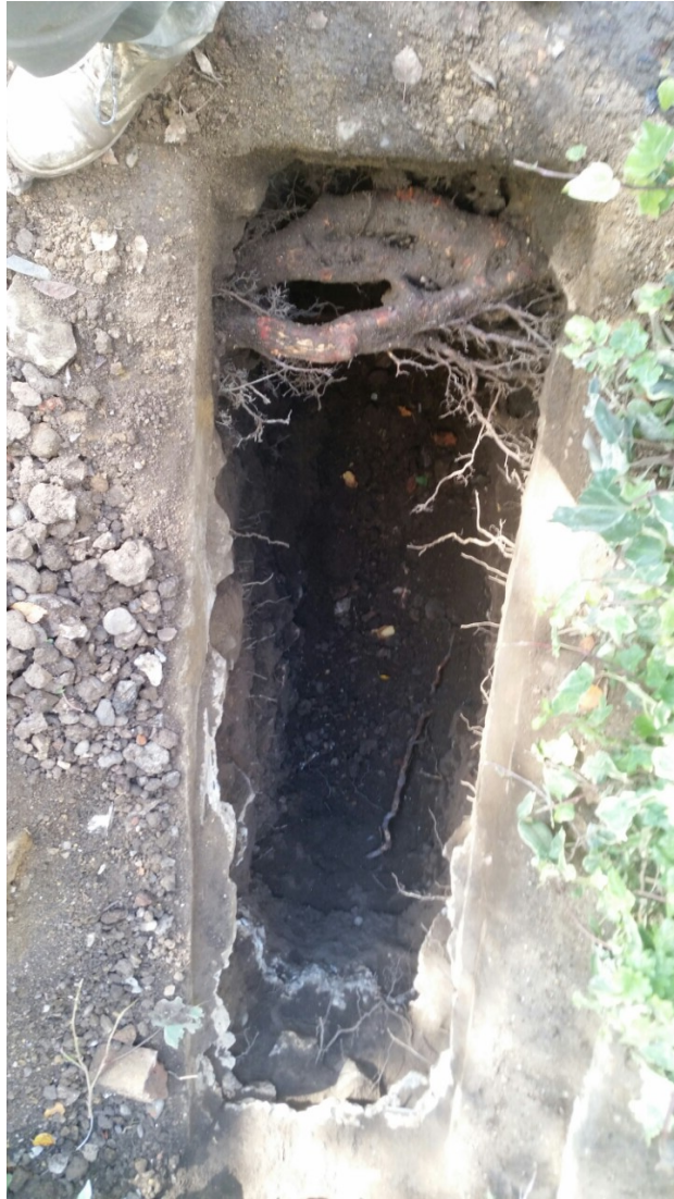
Photograph 3: Trial Pit 2 (200cm long 900mm deep) with Root 1 (120mm diameter at 100mm deep -measured at widest part before the root splits)
