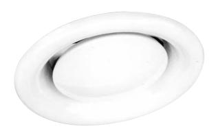
Valve adjustment is achieved by simply rotating the central core inwards or outwards on its spindle and locking into its set position using the holding nut at the rear of the valve assembly. The GXF Fire Rated Valve functions as a normal extract valve, sharing the same basic construction and performance as the GXD, however this unit also incorporates a spring
