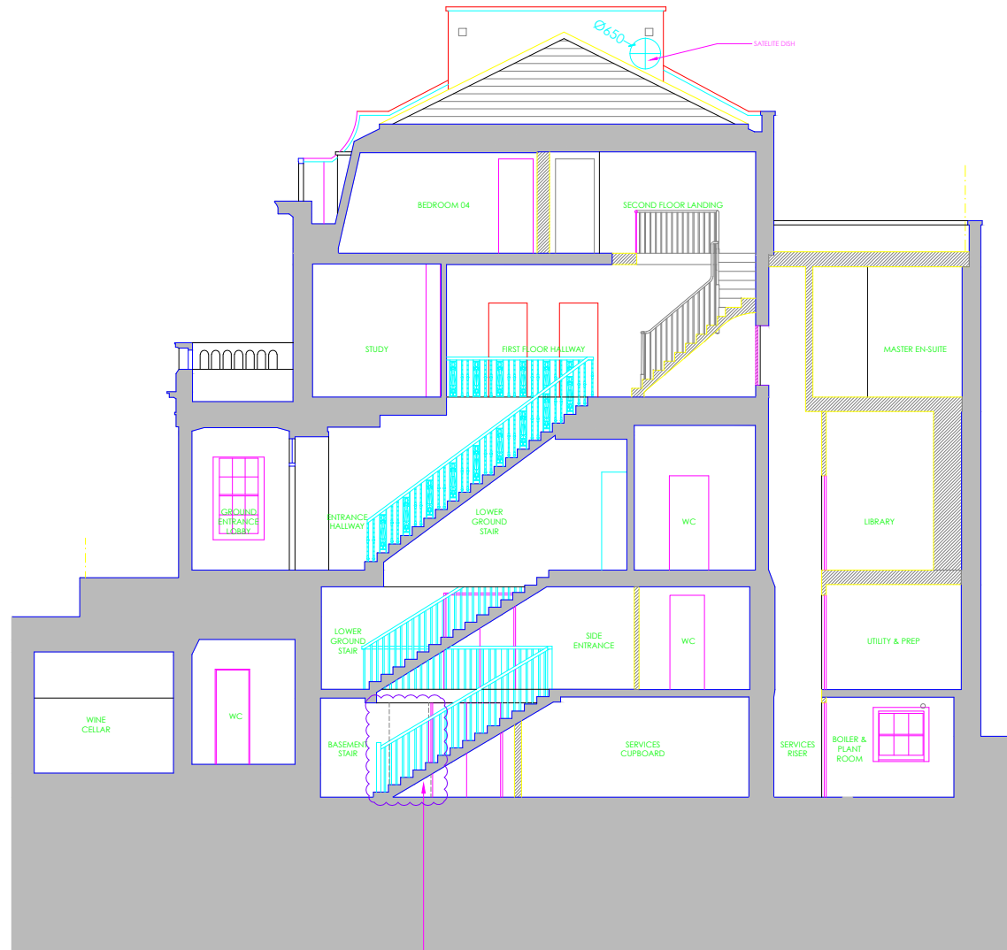
NEW DOOR OPENING INTO SNUG ACCESSED FROM HALL SHOWN IN GREY LINE SECTION K-K
