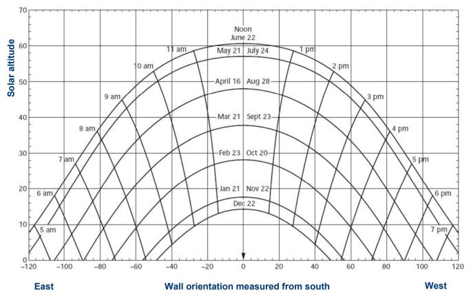
The proposed design has recessed glazing, where achievable, where the wall structures effectively work as horizontal overhangs and vertical fins. Vertical fins contribute to the reduction of unwanted solar gains occurring at low solar altitudes at West and East facades. In the South façade, the proposed design will benefit from passive solar gain in the winter when solar altitudes are low, also the horizontal overhangs will help reduce unwanted solar from high altitude sun in the summer.
