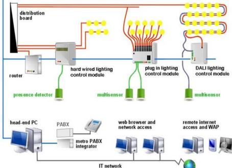
Changes to standards such as Part L Building Regulations, have pushed the standards for efficiency in lighting installations and promoted the use of lighting controls systems.
