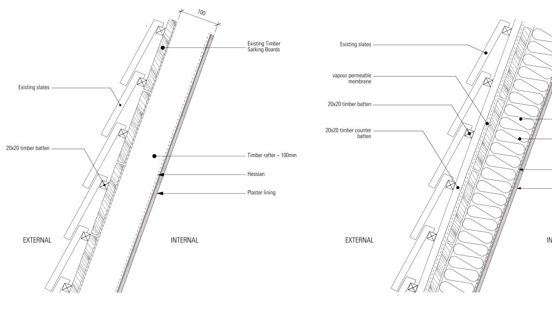
**A Existing Roof Insulation Detail with Internal finishes** Scale 1:5 @A3
