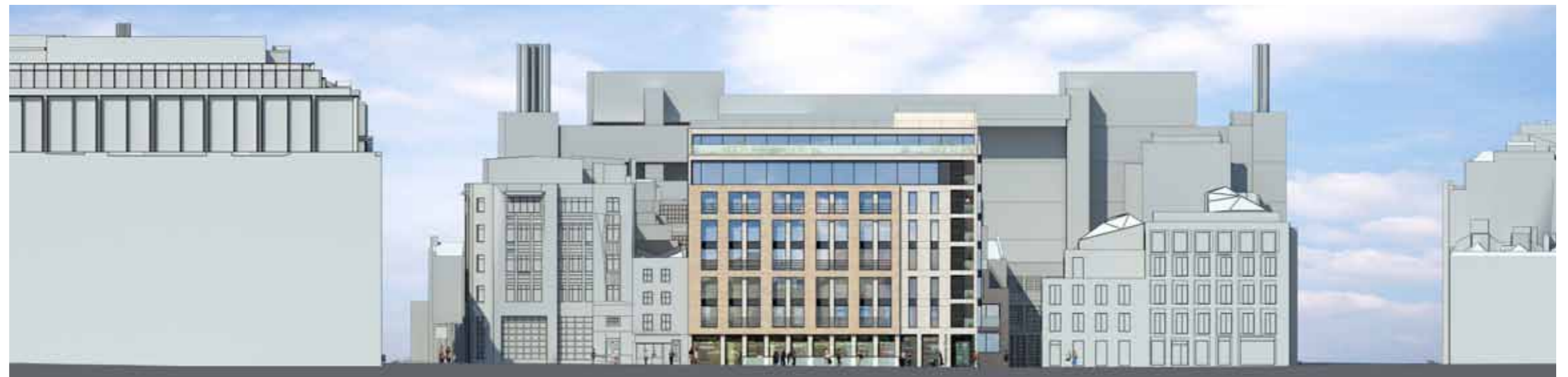
Figure 2.2.2. Tottenham Street facade - proposed approach 1 ( stepped approach to facade responding to key levels in adjoining buildings).
