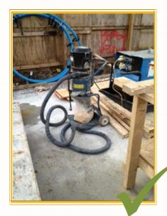
This hard wearing dust extractor attaches to most cutting saws. The bag system allows for large amounts of cutting without constant stopping to empty.
