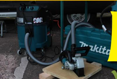
Chaser fitted to an industrial vacuum for use internally.
