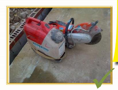
This unit attaches to the water suppression pipe on the grinder, it allows water to be pumped at a constant steady pace, allowing the spray to be supplied controlling the dust.
