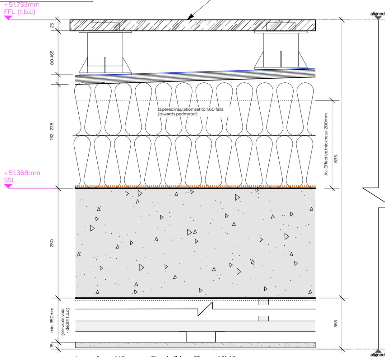
**Lower Ground / Basement Floor build-up: [External Slab]**
