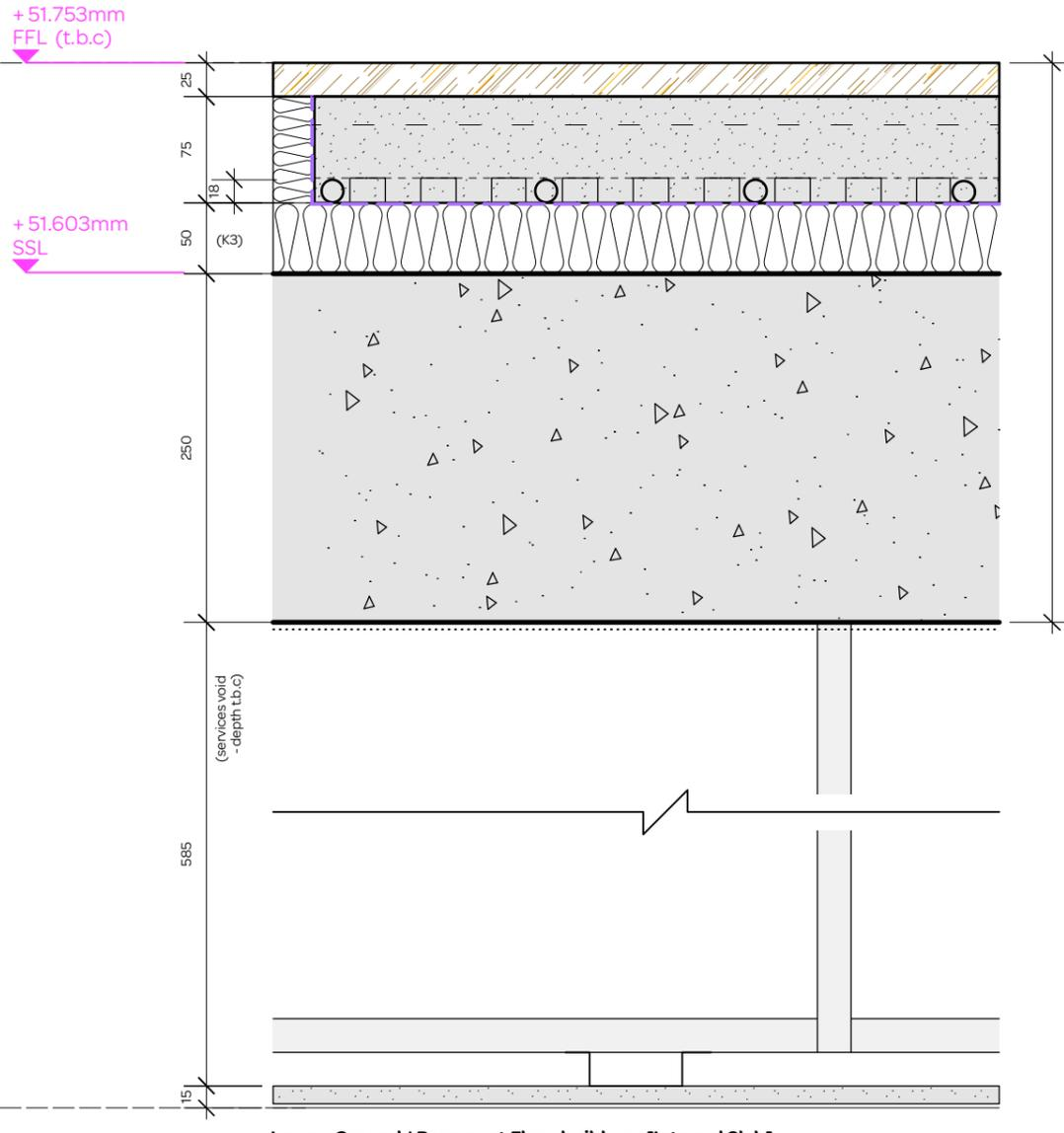
**Lower Ground / Basement Floor build-up: [Internal Slab]**
