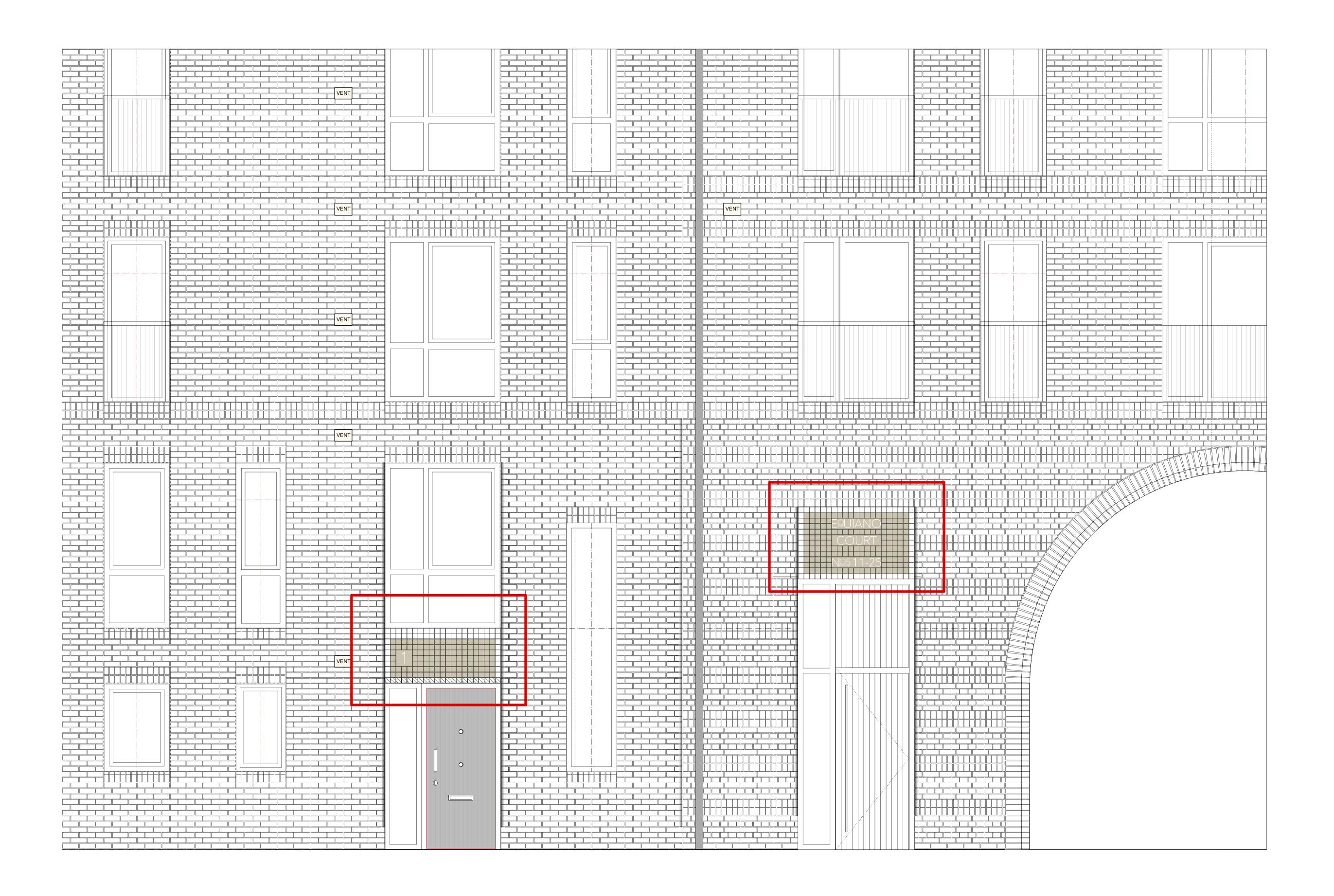
TYPICAL TILED SIGNAGE ARRANGEMENT - BLOCK 2 SOUTH ELEVATION SHOWN (PARTIAL) (others tiled signage similar - see GA elevations for locations & variations)
