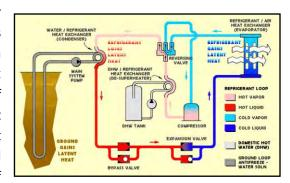
a heat pump, an air delivery system (ductwork), and a heat exchanger-a system of pipes buried in the shallow ground near the building. In the winter, the heat pump removes heat from the heat exchanger and pumps it into the indoor air delivery system. In the summer, the process is reversed, and the heat pump moves heat from the indoor air into the heat exchanger. The heat removed from the indoor air during the summer can also be used to provide a free source of hot water.
