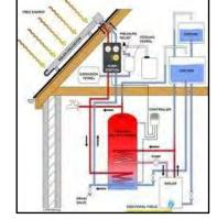
SWH systems in general have a 5-10 years warranty and require little maintenance. A yearly check by the owner of the system and a more detailed maintenance check by a qualified installer every 3-5 years should be adequate.
