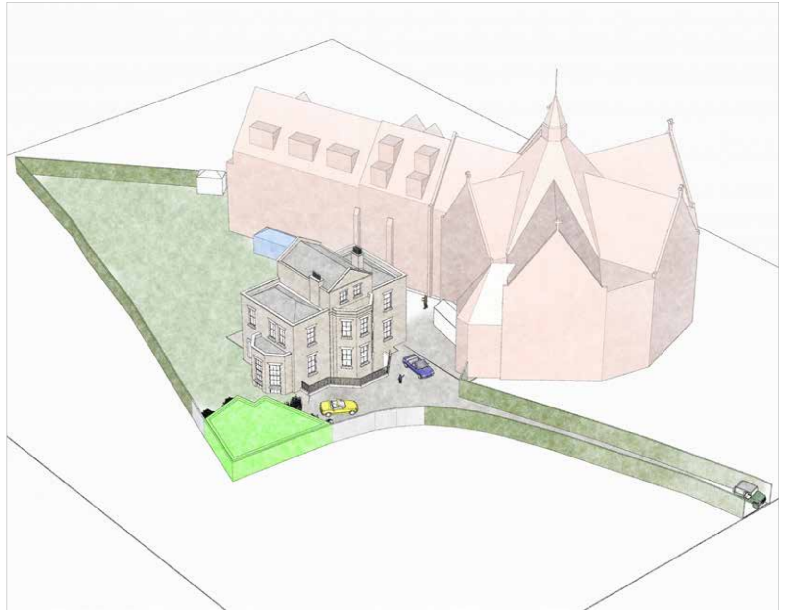
Existing view looking east, buildings to be demolished shown in blue, Studio to be converted shown in green
