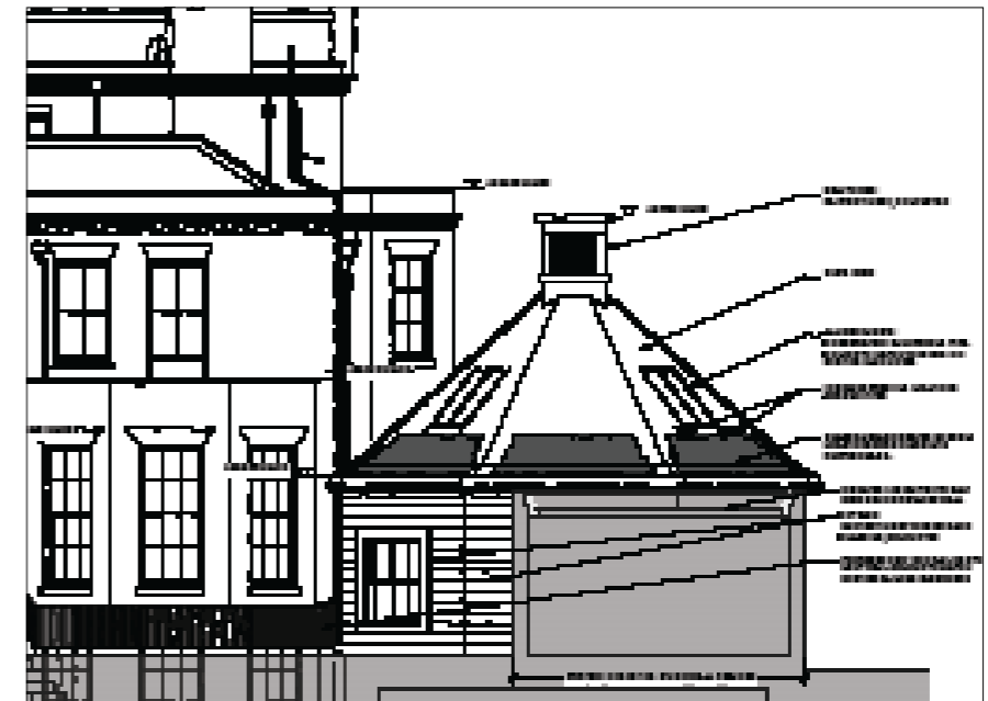
Partial elevation showing possible solar slate locations
