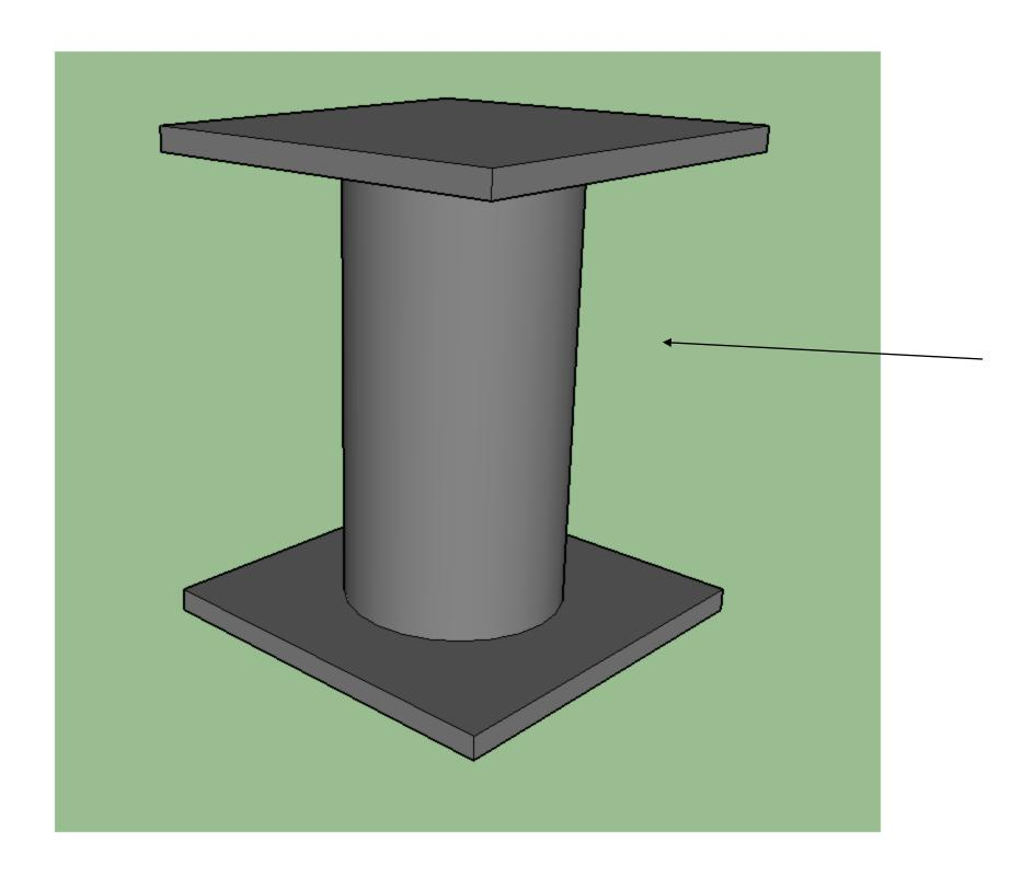
Existing Internal load bearing walls, steel stool installation. A continuous slot is created at the base of existing internal load bearing walls, using steel stools installed in an underpinning type sequence to provide temporary support to the walls
