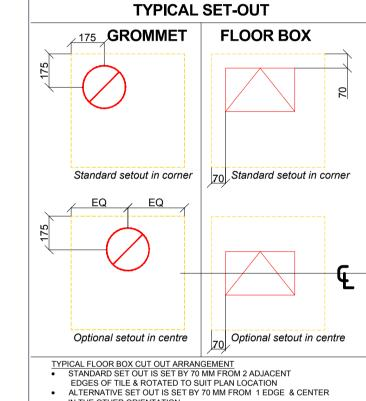
TYPICAL GROMMET CUT OUT ARRANGEMENT
