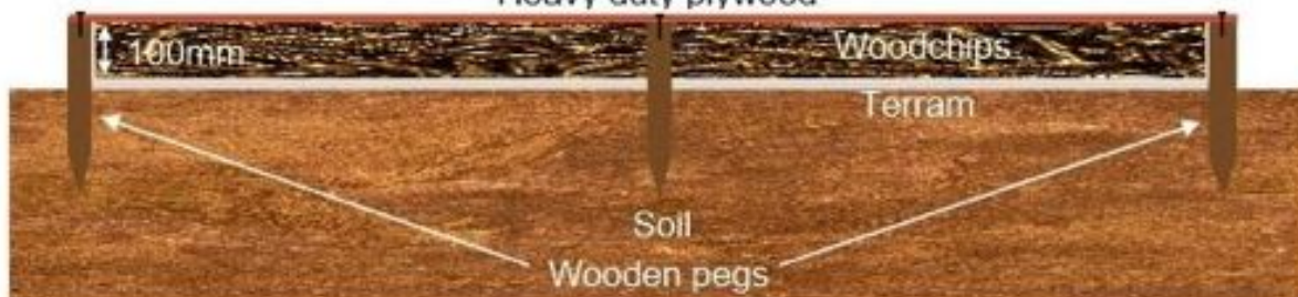
Figure 7. Plywood sheeting used as ground protection.
