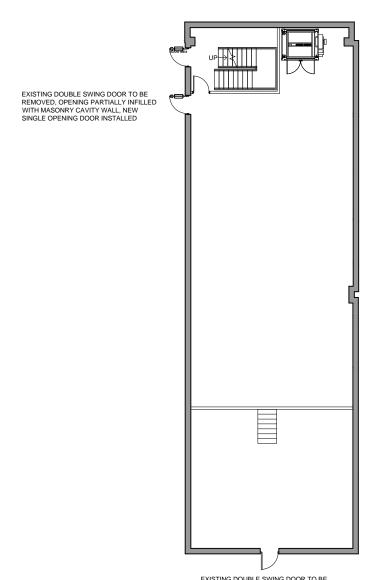
EXISTING DOUBLE SWING DOOR TO BE REMOVED, OPENING PARTIALLY INFILLED WITH MASONRY CAVITY WALL, NEW SINGLE OPENING DOOR INSTALLED
