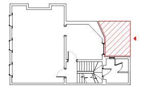
Line of parapet wall Red dotted lines indicate re-located condenser unit, below parapet wall Black dotted lines indicates recess behind parapet wall where existing condenser units are sited
