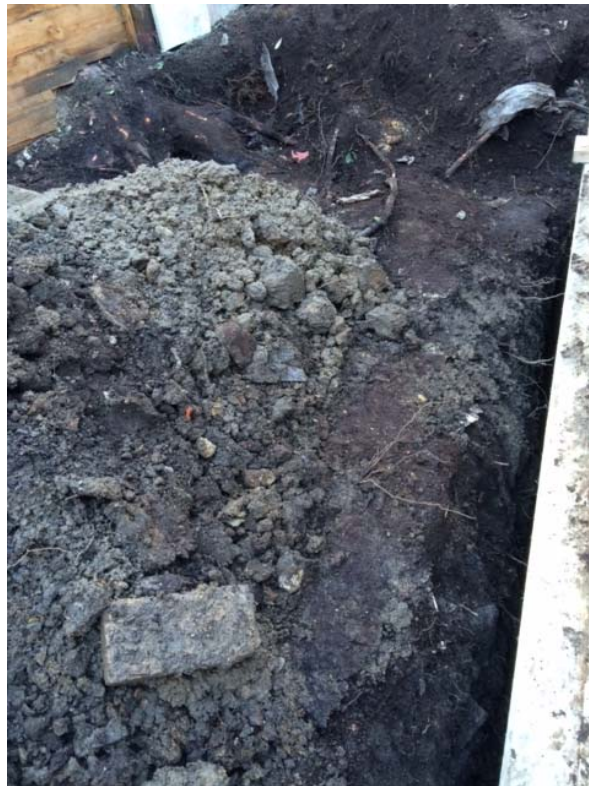
Photograph 2: Trial Pit 1 (trench 2m long and 700mm deep) only fibrous roots discovered
