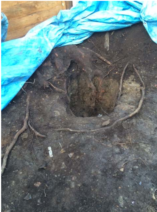
Photograph 3: Trial Pit 2 (300mm deep) showing surface buttress root growing straight down at this point
