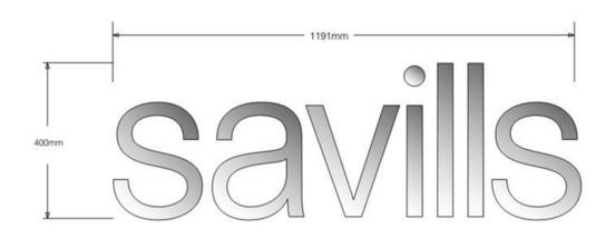
Built up brushed stainless steel letters each letter to have internal white led illumination to give halo glow around letters. All letters electric link cables to go through rear panel (I.E. To hide cables) transformer mounted internally.
