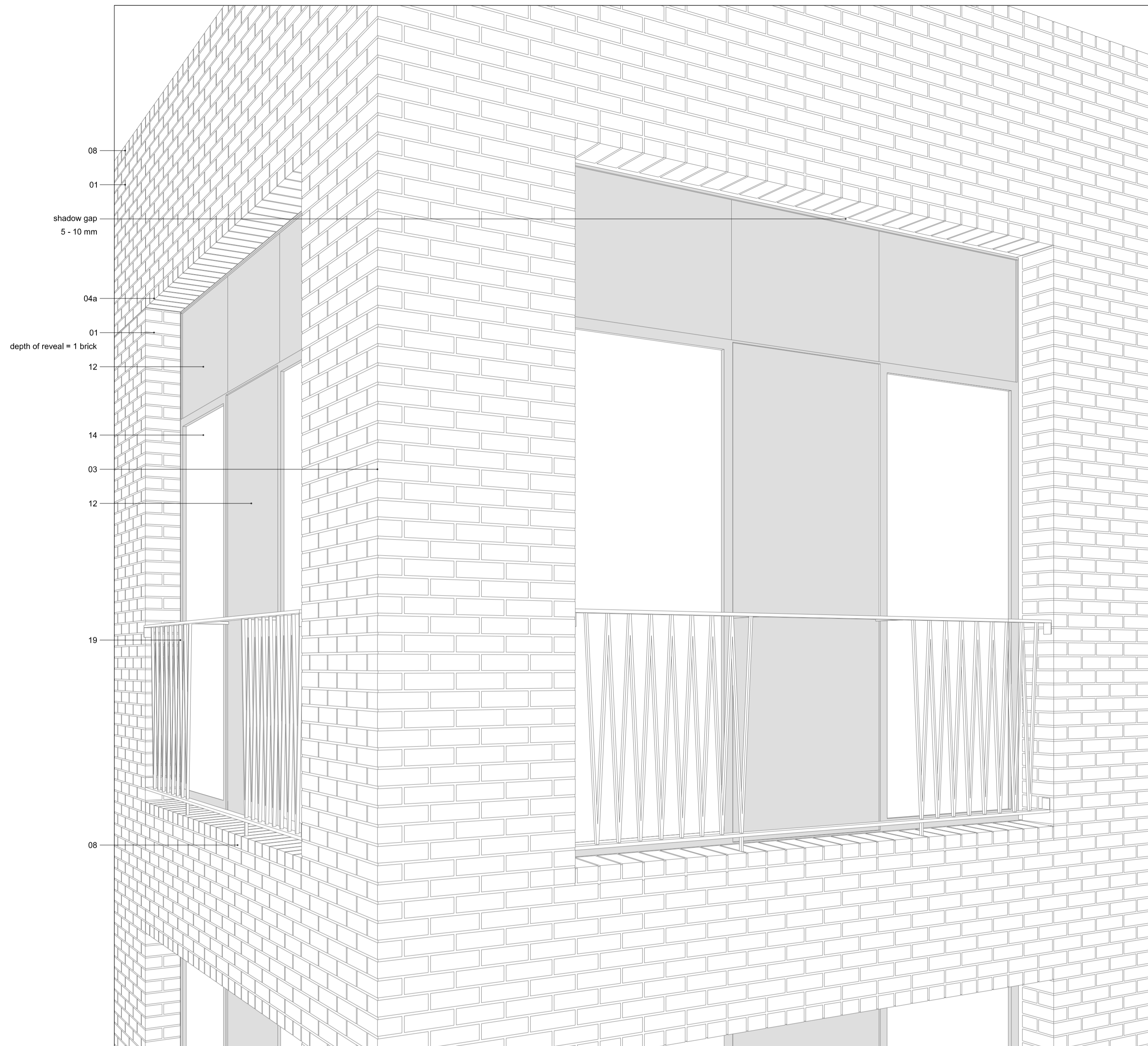
Illustration of typical 2nd floor opening at the bookends with panels above windows
