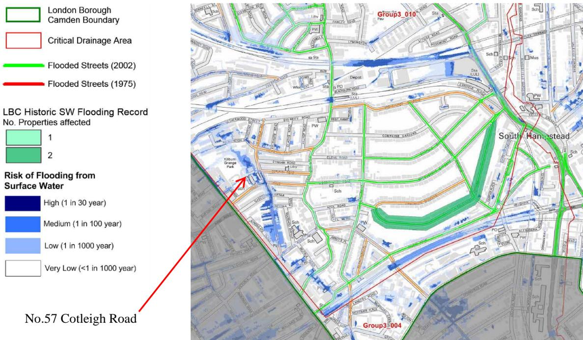
**Figure 9:** Extract from Figure 3v of the Camden Strategic Flood Risk Assessment (SFRA) (URS, July 2014) showing risk of flooding from surface water.
